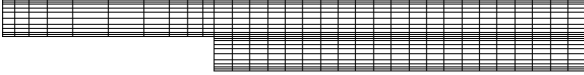
Figure 3.5 – Backward-facing step entrance and a portion of the separation region of mesh
